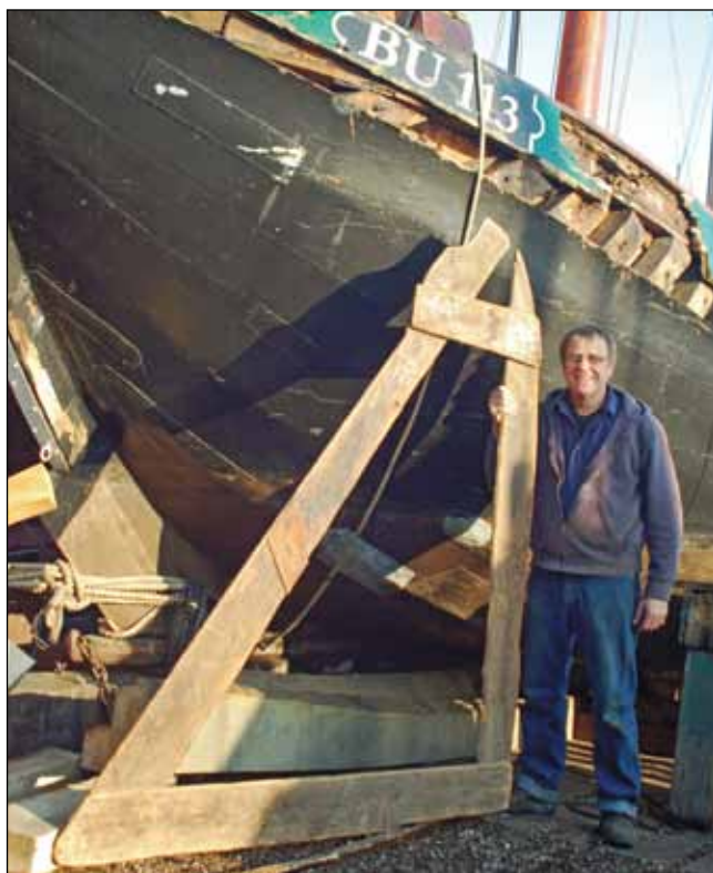
Botters are built using patterns handed down through generations, like this Nieuwboer rudder pattern, held by Nieuwboer manager Henk van Halteren. This pattern has been in use since 1842.
